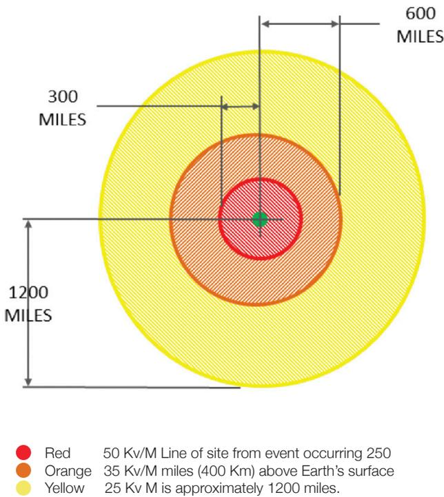
\*Simulated blast configuration of 400 km altitude (above), not only taking into account Earth's magnetic field. A low altitude event would only show effects approximately 15 km. HEMP event over Kansas would affect ICs in systems from California to New York.
