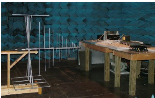
Radiated Emissions Test Setup
