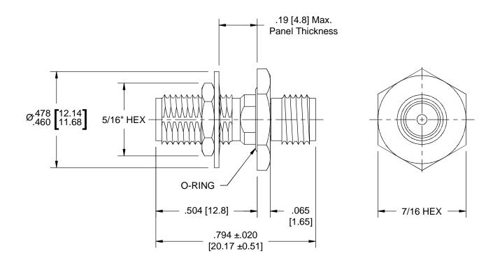
Panel Nut, Lock Washer and O-Ring are Shipped Unassembled.
