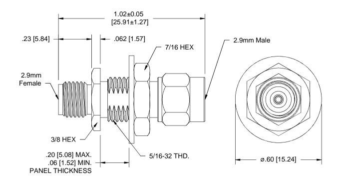
NOTE: COUPLING NUT, RETAINING RING, PANEL NUT AND LOCKWASHER ARE SHIPPED UN-ASSEMBLED.
