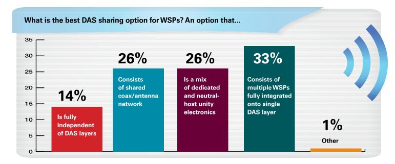
"The most efficient option for WSPs in key strategic high wireless traffic areas is to have a neutral host system wherein multiple carriers with multiple technologies can be delivered through a shared fiber backbone and supporting nodes. Otherwise, you lose the efficiency of space by having redundant single dedicated systems for each WSP," says Grimes.
