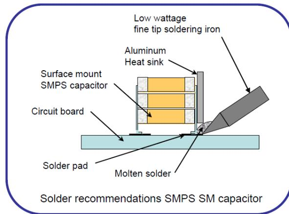
After soldering is completed, assemblies should be allowed to cool naturally to room temperature. If an oven was utilized for the purpose of preheating the assembly, the circuit
